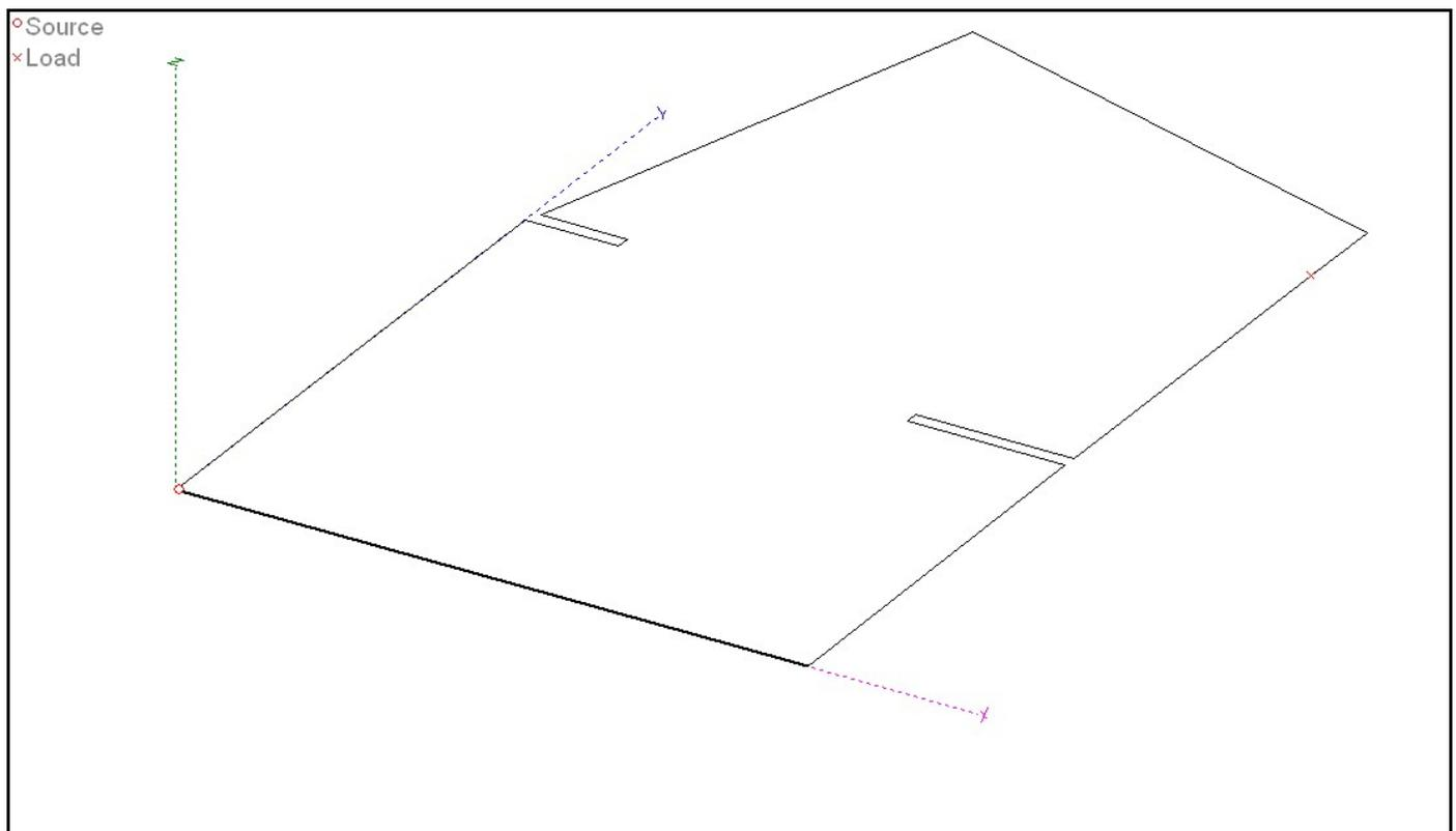
antenna layout / circumference about 30m / source in lower left (matched to 50 Ohm by a 1:22 balun), 1k terminator at the opposite side / the two indentations have no technical meaning but are simply because of walls that I did not want to drill holes into (HI)
